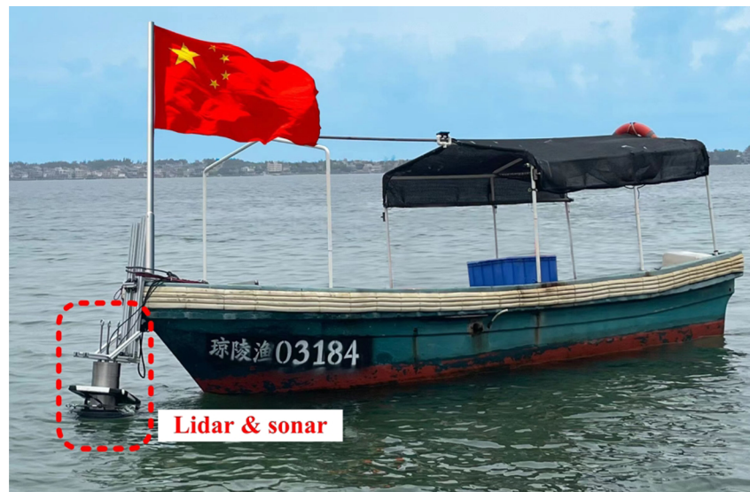
Fig. 4. Picture of the shipborne single-photon underwater lidar during the field experiment.
